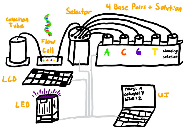
Figure 4: Integration of Entire System
